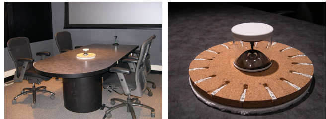
Fig. 1. Smart Room. The left figure shows the smart room. The right figure shows the microphone array and the omnidirectional camera.
