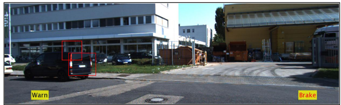
Both Warning & Brake Alert are issued, a high acceleration was found in an abrupt left turn.
