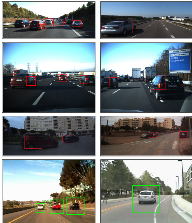
Figure 2: Results of on-road vehicle detection
