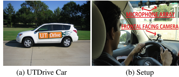
Fig. 1. Car platform used for the recording. (a) picture of the UTDrive car (b) placement of the frontal camera and the microphone array.
