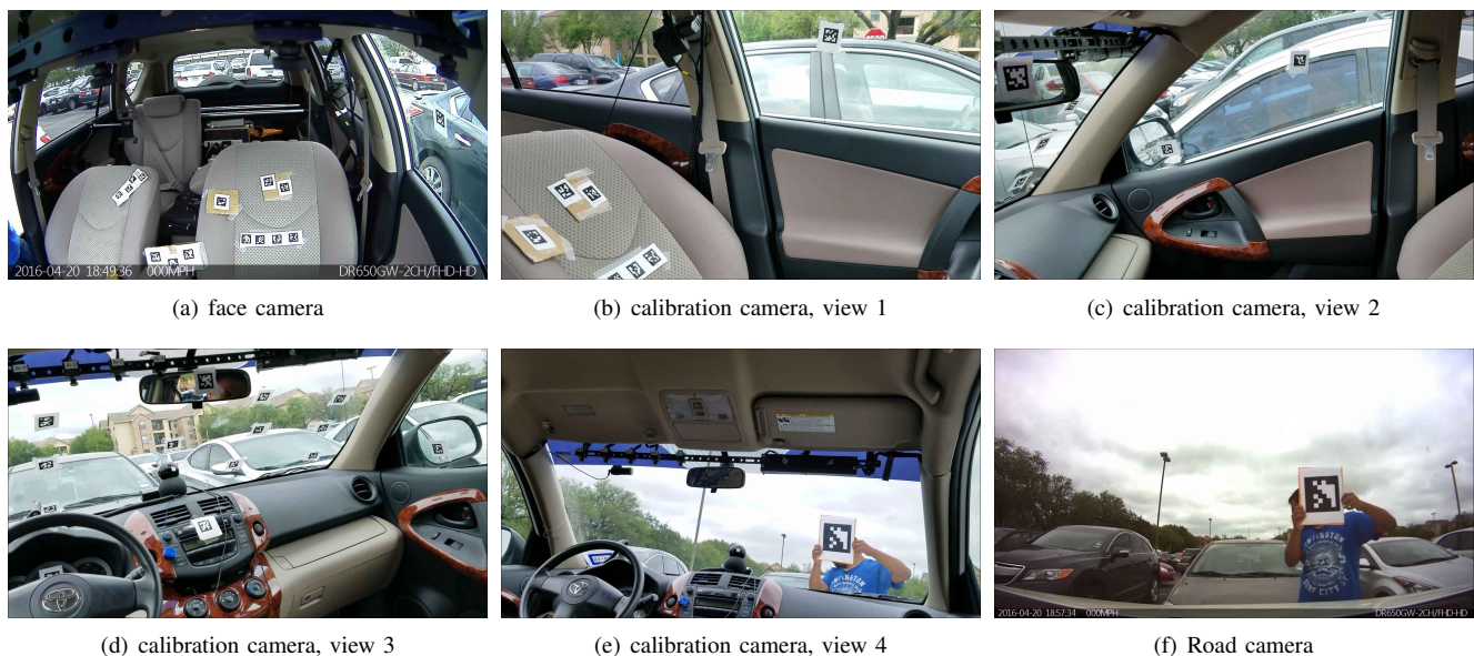
Fig. 5. Description of the process to calibrate the cameras and define a common reference system. Figures (a)-(d) show the calibration for the markers' locations and the face camera. Figures (e)-(f) show the calibration for the road camera.
