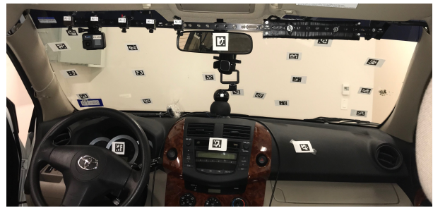
Fig. 7. We place AprilTag on top of the target markers to estimate their exact position in the 3D space during the calibration.
