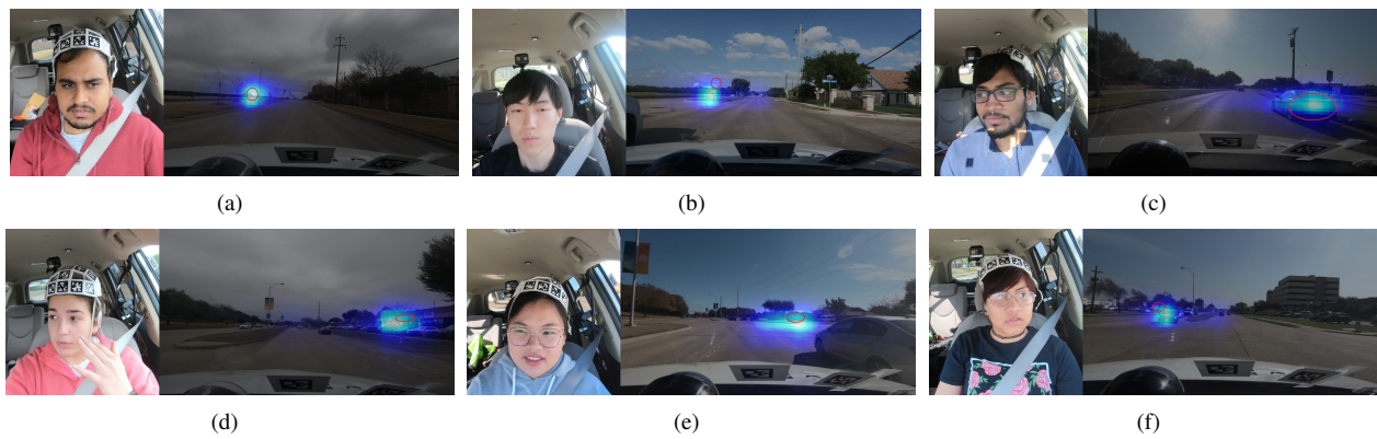
FIGURE 16. Examples of road projection of the visual attention estimation where the ground truth overlaps with the model estimation. The red circles indicate the target gaze direction. The figure is best viewed in color.
